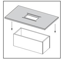
3. Apply 4 x pea sized dabs of silicone to the table top, close to the burner cut out.
