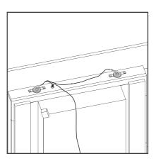
Insert a packer behind the fire to firmly push the fire and the back panel against the body.
