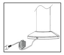
3. Feed the cable through the groove out of the base.
