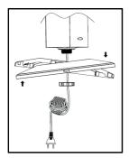
Snap the 2 halves of the base together and pass the power cord through the centre hole of the base.
