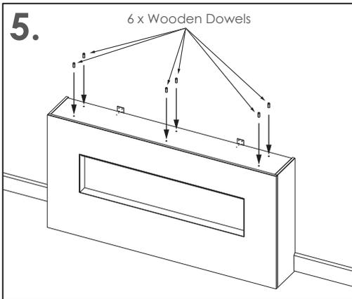
**5.** Insert 6 x dowels into the holes on top of the base.
