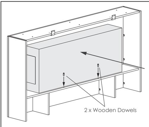
Insert the fire into the base, pushing the fire into the cut out.
