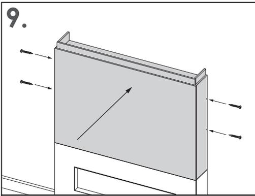
**9.** Keep the top box pressed firmly against the wall. Then, using the 4 x large screws provided, screw into the pre-drilled holes in the side of the top box to fix the top box in position.
