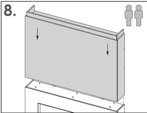
**8.** With help, carefully lift the top box then lower and sit the top box onto the dowels on top of the base.
