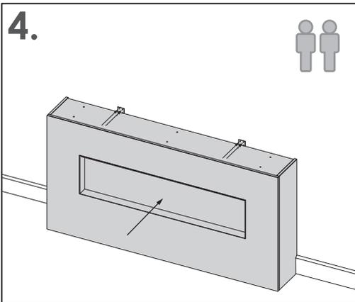
**4.** Position the base against the wall and, using the appropriate fixings, secure the brackets to the wall.
