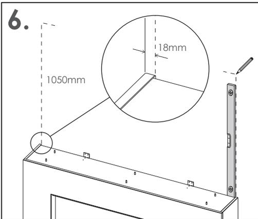
**6.** Using a spirit level so the lines are straight. Measure 1050mm from the top of the base and mark a line 18mm inward of the outer face of the base on the wall. Do this on both sides of the base.
