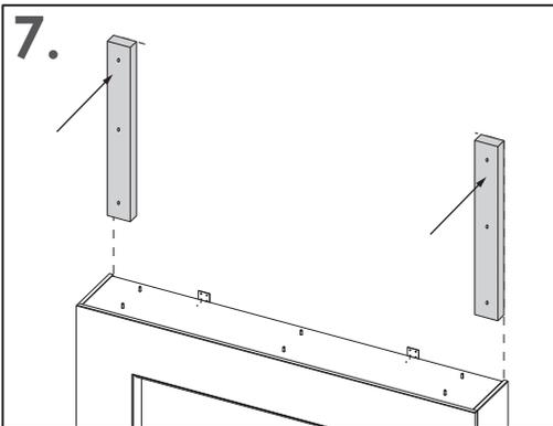
**7.** Using the appropriate fixings, securely fit 2 x timber battens to the inside of the lines marked on the wall.
