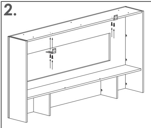
**2.** Using the 4 x small screws supplied, turn the brackets from the fire around and fix to the **UNDERSIDE** of the base top. Use the pilot holes to locate the brackets.
