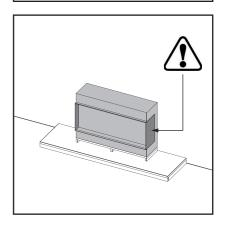
With help, lift the body onto the hearth and push back against the wall, ensuring the fire slides into the opening.
