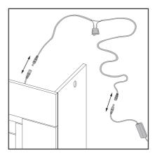
7. Detatch the switch from the extension cable and insert the switch into the hole in the leg, then re-attach the cable to the switch.
