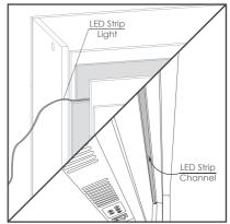
Once the LED strip lights are fitted, connect the extension cable to the LED strip lights and the plug driver cable to the extension cable.
