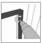
3) Attach the spacer to the surround using 8 x (3.5 x 12mm) screws or similar size 4) Offer the fire up to the spacer. Check the supply cord is not trapped under the fire such that it may cause it to be damaged.
