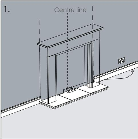
1. Make the relevant cuts to the skirting board to accommodate the width of the fireplace body.
