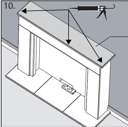
Using 'pea sized' dabs of silicone, adhere the underside of the shelf to the chamber back panel & sides.
