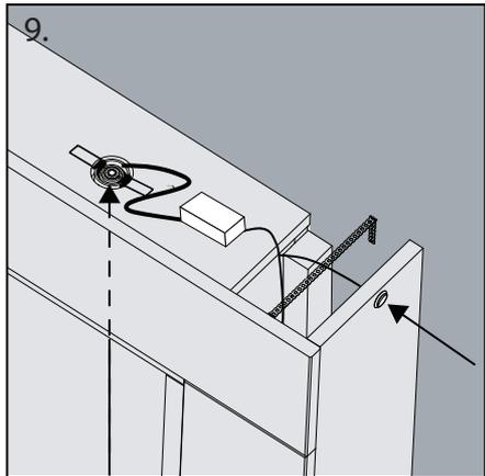
9. Insert the down lights and connect the switch to the right leg.
