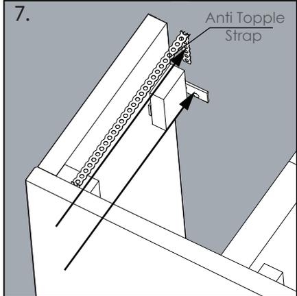
6. Position the fireplace body and fix to the wall using the anti-topple straps and brackets provided, as shown in Illustration 7.
