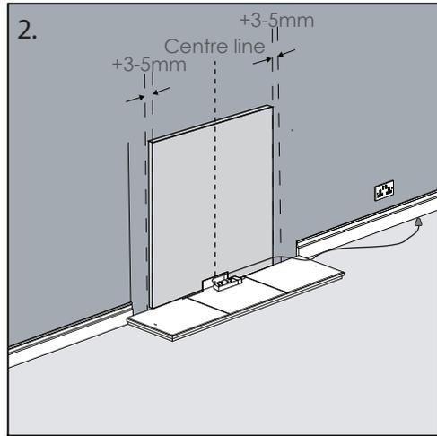
2. Measure the chamber back panel & add 3 to 5mm to each side. Mark this line on each side.
