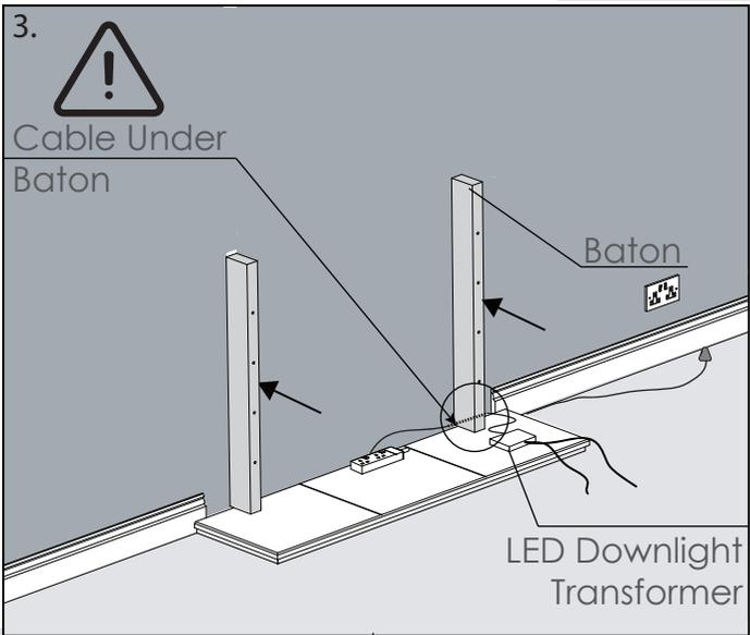
3. **Warning:** Prior to baton fitting, obtain the LED downlight set and plug into the extension. Feed the rest of the cable behind the hearth towards the cable side, underneath the baton.
