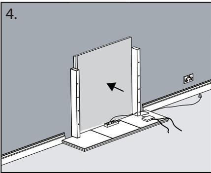
4. Using appropriate marble adhesive, adhere the chamber back panel flat to the wall, leaving an even gap between the 2 fixed batons. Ensure the extension sockets are fed through the cut out of the back panel.
