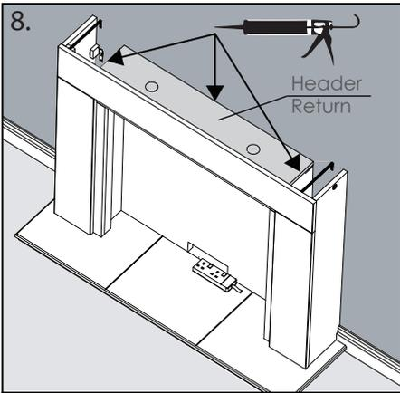
8. Using 'pea sized' dabs of silicone, adhere the header return to the chamber back panel & sides
