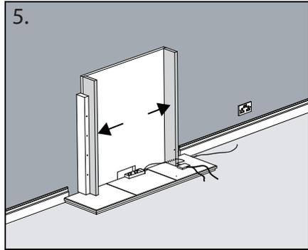
5. Using the appropriate marble adhesive, adhere the chamber sides to the batons ensuring the sides are pushed up tight to the back panel.
