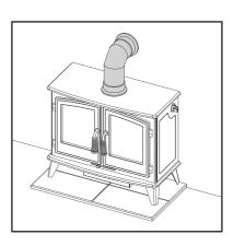
4. To position the split batten, measure a MINIMUM distance of 75mm from the top of the stove pipe to the bottom of the split batten and mark the wall.
