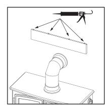
6. Slide the beam over the batten and lower into position.
