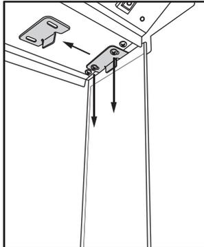
5. Remove the 2 x screws from the bracket holding the side glass in place.
