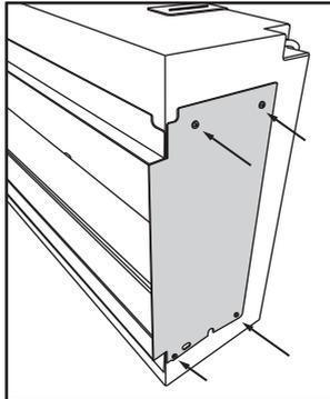
8. Replace 4 x screws into the holes in the side of the fire to fix side panel.
