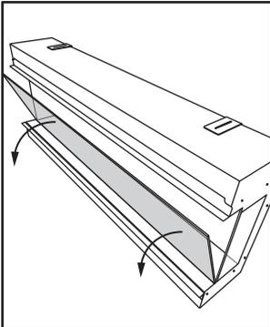
4. Carefully tilt the front glass forward and lift to remove.
