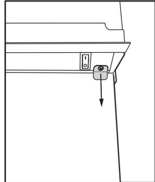
3. Remove the screw from both brackets on the front of the fire to remove the front glass.
