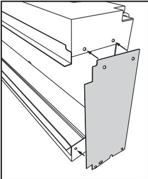
7. Position the side panel so the holes line up with the holes on the side of the fire.
