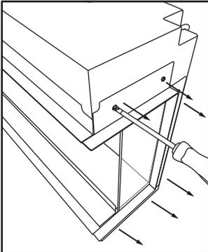
1. Remove 6 x screws from the side of the fire
