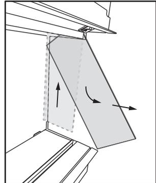
6. Carefully lift and tilt the side glass and remove.
