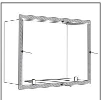
Fix the fire in position, central to the opening, from the rear.
