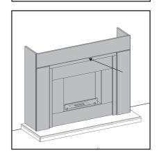
Once in position, fix the body to the wall using the anti-topple straps and the brackets provided.
