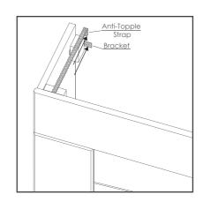
Once brackets are in place, apply 3 x "pea sized" dabs of silicone onto the top edge of surround and, with help, lift the shelf and slowly lower onto the surround.
