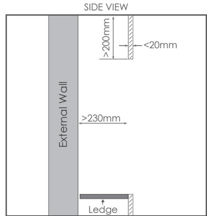
Behind the wall, a ledge must be positioned at the bottom of the opening for the firebox to sit on.
