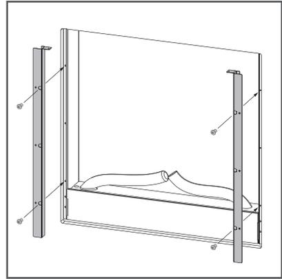
4. Once flat against the wall, use 4 x screws to secure the Firebox in place.
