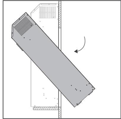
3. Once in the wall, locate the 2 x fixing brackets and fix to the firebox using 4 x screws removed from the metal tabs.
