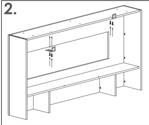
Using the 4 x small screws supplied, turn the brackets from the fire around and fix to the **UNDERSIDE** of the base top. Use the pilot holes to locate the brackets.
