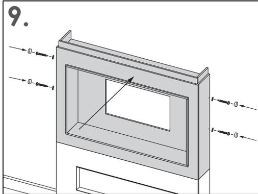
Keep the top box pressed firmly against the wall. Then, using the 4 x large screws provided, metal screw cap washers and 4 x the pre-drilled holes, drill into the timber battens fixed to the wall.
