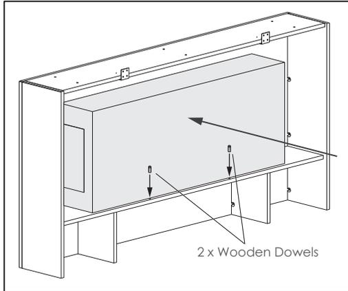
Insert the fire into the base, pushing the fire into the cut out.
