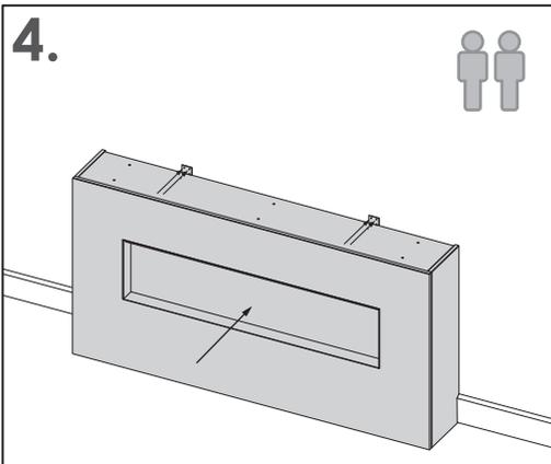
Position the base against the wall and, using the appropriate fixings, secure the brackets to the wall.
