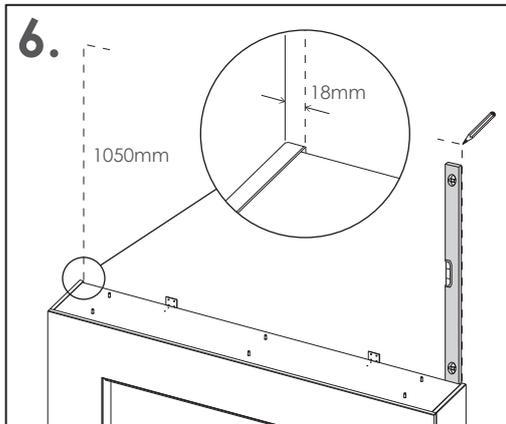
Using a spirit level so the lines are straight. Measure 1050mm from the top of the base and mark a line 18mm inward of the outer face of the base on the wall. Do this on both sides of the base.
