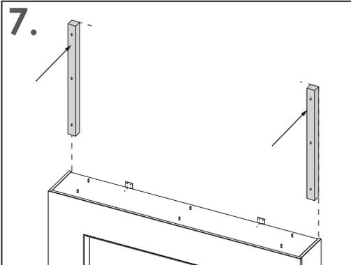
Using the appropriate fixings, securely fit 2 x timber battens to the inside of the lines marked on the wall.
