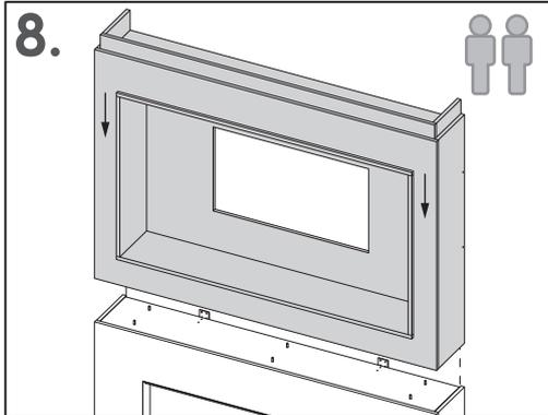
With help, carefully lift the top box then lower and sit the top box onto the dowels on top of the base.
