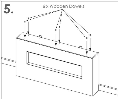
Insert 6 x dowels into the holes on top of the base.
