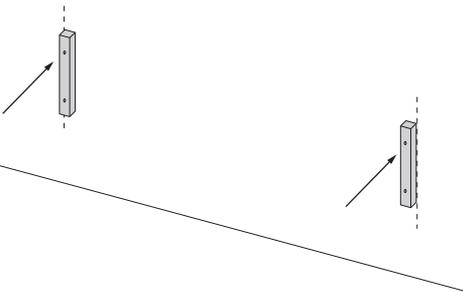
Using the appropriate fixings, securely fit 2 x timber battens to the INSIDE of the lines marked on the wall.
