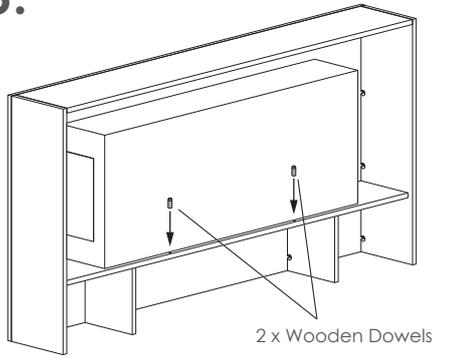
Once in position, Insert 2 x dowels into the shelf to secure the fire.
