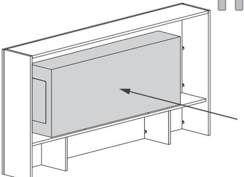
Insert the fire into the product and push the fire into the cut out .
