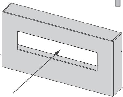
Before the fire is fitted, push the product against the wall in the desired position.
