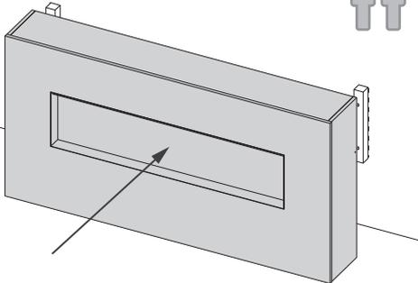
With help, carefully move the product back against the wall using the 2 x timber battens to guide it back into the chosen position.
