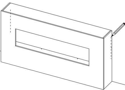
Lean through the cut out for the fire and mark the inside of both sides on the wall using a pencil. These lines show where the battens are to be fitted.
