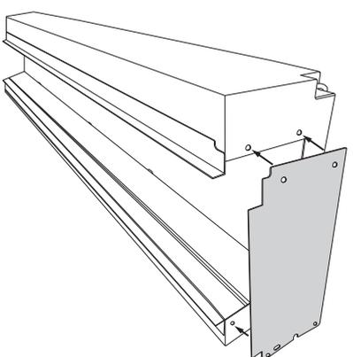
Following the instructions provided with the metal side panels, attach the metal side panels to the fire.
