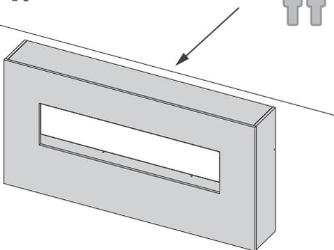
Move the product off the wall and place on the floor, ensuring there is enough room to access the back in order to fit the fire.
