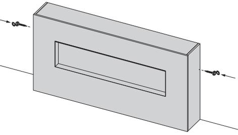
Keep the product pressed firmly against the wall. Then, using the 2 x large screws provided, screw caps and 2 x the pre-drilled holes, drill into the timber battens fixed to the wall to secure the product.
