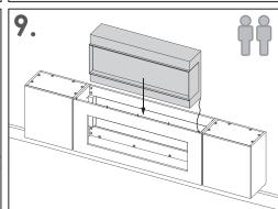
With help, lift the fire and carefully place it inside the fire unit.
