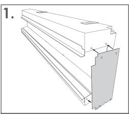
Following the instructions provided with the metal side plates, attach the side plates to the fire.
