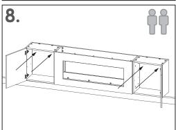
Using an appropriate fixing method, fix the cupboards to the wall for added strength and security.
