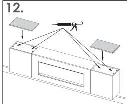
Using the fire unit worktop as a reference, fix the cupboard worktops to the cupboards using an appropriate adhesive.
