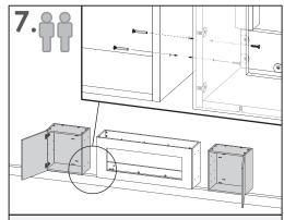
With help, one at a time, line up the cupboards with the fire unit. Keep these lifted/supported and ensure they are level with the fire unit. Fix the cupboards to the fire unit using the connecting screws and screw sleeves provided.
