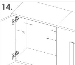
Insert the shelf pegs into the pre-drilled holes at the desired height in both cupboards.
