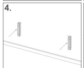
Place the fire unit on the floor and, using the appropriate fixings, securely fit 2 x Short Timber Battens to the INSIDE of the lines marked on the wall.
