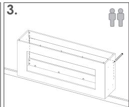
With help, hold (or prop) the fire unit against the wall at the chosen height. Ensure the fire unit is level and using a pencil, mark the inside both sides and under the top support on the wall.
