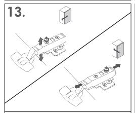
Now the worktops are on, using a screwdriver, adjust the hinges on the cupboards to ensure the doors are square and level.
