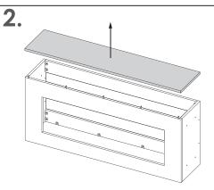
Remove the worktop from the fire unit by carefully lifting the worktop upwards.
