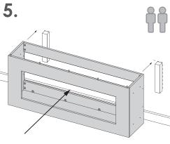
With help, lift and hang the fire unit on the battens.
