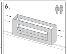
Keeping the fire unit pressed firmly against the wall, use 4 x Large Screws to fix the product to the battens through the pre-drilled holes.
