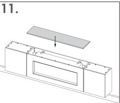
Fix the fire unit worktop back onto the dowels on the fire unit
