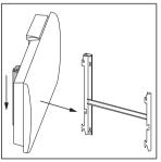
2. Push the bracket down and remove from the hooks.
