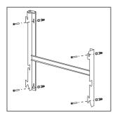
3. Place the bracket against the wall, ensure it is level and mark the 4 holes on the wall.
