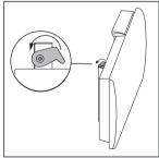
1. Loosen the screw (do not remove) and turn the security clip to release the bracket.
