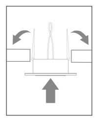
2. Holding the spring clips up, insert the down light in to the holes and release.
