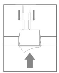
3. Release & join the connectors as shown to install switch.
