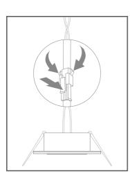
1. Release & join the connectors as show to install down light.
