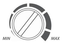
Please note that the appliance can only be switched on when the thermostat setting is higher then the room temperature.
