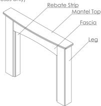
Please identify the parts listed below and ensure you have **ALL** the correct parts before assembling the unit.
