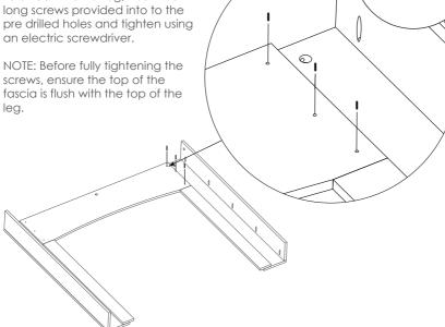
2. Repeat step 1 with the other leg, again ensuring the top of the fascia is flush with the top of the leg before fully tightening the screws.
