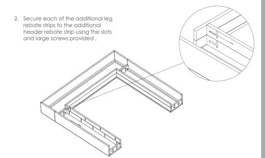
**IMPORTANT:** KEEP THE ADDITIONAL REBATE STRIP SET AND THE FIXING SCREWS IN A SAFE PLACE AS THEY MAY BE NEEDED SHOULD A DIFFERENT REBATE SIZE BE REQUIRED.
