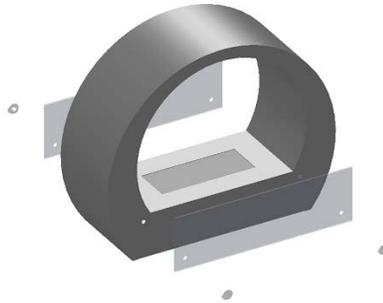
2. Place the burner into the burning chamber of the fireplace body.
