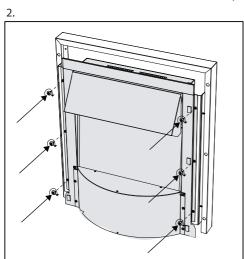
Attach inset fire to spacer, using self tapping screws provided, & screw driver.
