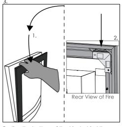
Postion the bottom of the trim behind the locating brackets on the fire, push the trim forward at the top, and then drop down, ensuring the fire locates within the corners of the trim. Then push down.
