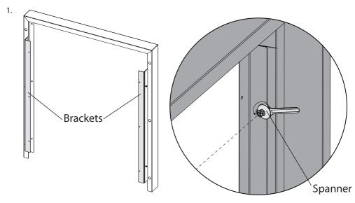
Ensure two brackets are fastened loosely, not tight. If tight, loosen with spanner provided.
