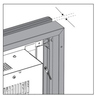
From the rear, adjust the trim and close any gaps, then tighten all 4 bolts.
