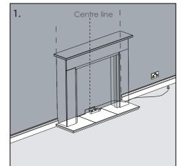
Make the relevant cuts to the skirting board to accommodate the width of the fireplace body.
