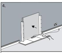
Using appropriate marble adhesive, adhere the chamber back panel flat to the wall, leaving an even gap between the 2 fixed batons.
