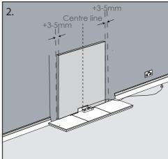
Measure the chamber back panel & add 3 to 5mm to each side. Mark this line on each side.
