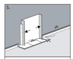
Using the appropriate marble adhesive, adhere the chamber sides to the batons ensuring the sides are pushed up tight to the back panel.
