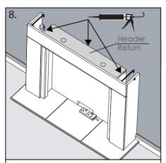
Using 'pea sized' dabs of silicone, adhere the header return to the chamber back panel & sides
