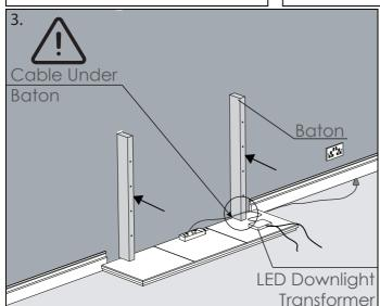
Prior to baton fitting, obtain the LED downlight set and plug into the extension. Feed the rest of the cable behind the hearth towards the cable side, underneath the baton.
