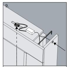
Insert the down lights and connect the switch to the right leg.
