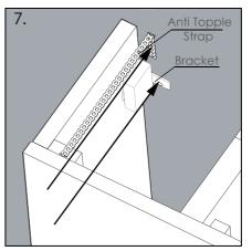
Position the fireplace body and fix to the wall using the anti-topple straps and brackets provided, as shown in Illustration 7.
