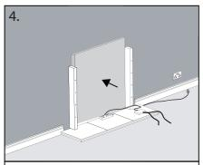
Using grab adhesive, adhere the chamber back panel flat to the wall, leaving an even gap between the 2 fixed batons. Ensure the extension sockets are fed
