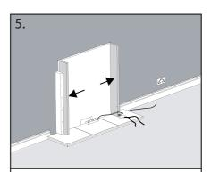
Using grab adhesive, adhere the chamber sides to the batons ensuring the sides are pushed up tight to the back panel.
