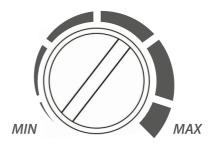
Please note that the appliance can only be switched on when the thermostat setting is higher than the room temperature.
