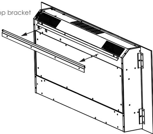
8. Align hole on the bottom bracket to the bottom of fire and mark the hole on the wall
