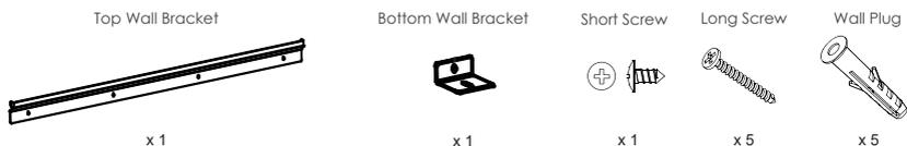
Note: Wall plugs supplied are for a solid wall. If screwing in to plaster board or wood, please use correct fixings.
