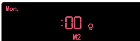
Press the time setting button
