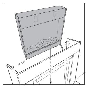
7. Once brackets are in place, apply 3 x "pea sized" dabs of silicone onto the top edge of surround and, with help, lift the shelf and slowly lower onto the surround whilst ensuring hooks go into brackets so the shelf is stable and does not move.
