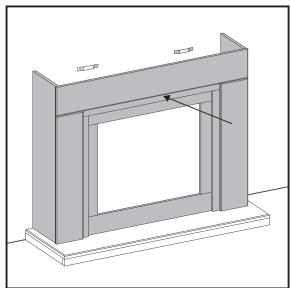
3. Once in position, fix the body to the wall using the anti-topple straps and the brackets provided.
