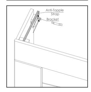
4. Take Firebox out of packaging and remove 4 x screws and brackets.
