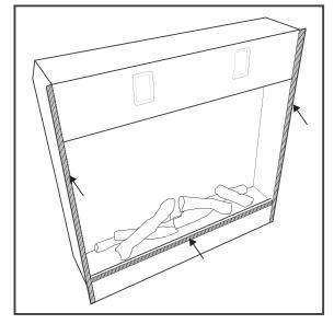
6. With help, lift the Firebox and feed plug into the surround, plugging it in whilst raised off the floor.
