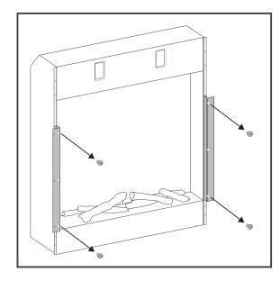
5. Fix the included neoprene strips along the length of the sides and bottom edge of the Firebox and remove the non-stick layer, exposing the adhesive.
