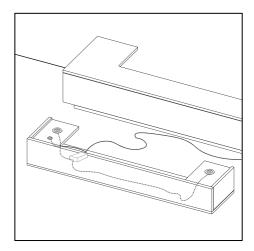
Before fitting the fire, move the downlights cable to the back, so the fire does not trap it.
